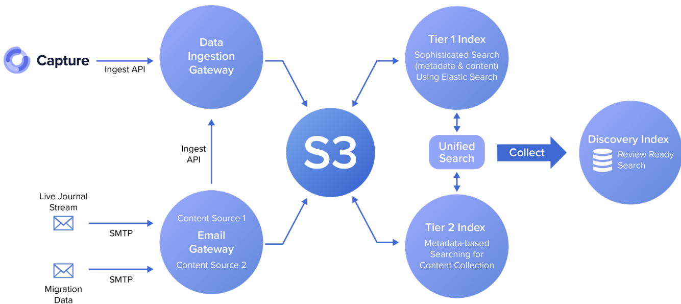
Figure 2. The Enterprise Discovery application enables a single query to collect data from both the primary and secondary tiers, and then automatically perform Index on Demand when the search results are collected into a case.
